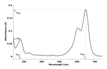
An absorption spectrum of a labeled antibody contains a dye peak (with a longer wavelength) and an antibody peak (at around 280 nm). The dye-to-antibody ratio is calculated using the following formula:
